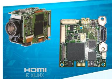
TWIGA provides a compact interface board that converts the native LVDS format from Tamron MP1010M-VC & new MP1110 camera zoom module.
