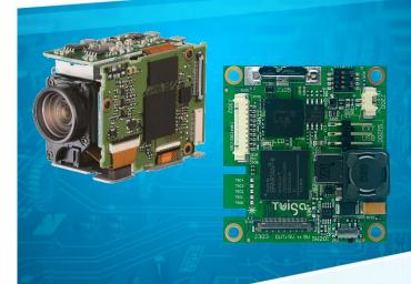
Twiga provides a compact USB3.0 interface board for Tamron MP1010M-VC module.
